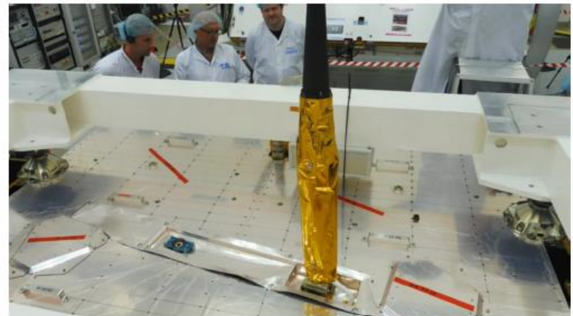
FM1 after successful boom deployment test
