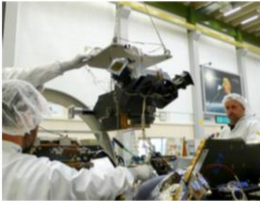
ACC/STR/TMA Integration On FM1 with nominal shims
