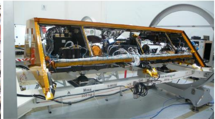
FM1 prepared for post-environmental alignment measurements
